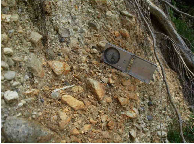
堆積面の走向傾斜N40W,20S
