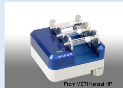
▲ Rotational floating culture system for 3D culture of iPS cells, etc.
