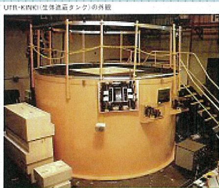
Biological shield tank of UTR-KINKI
